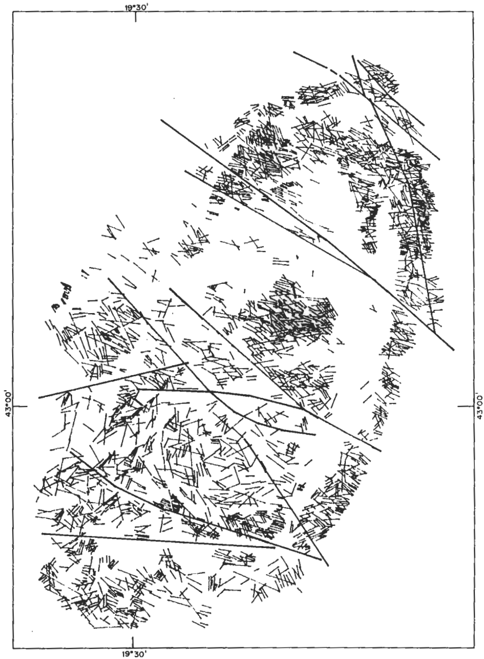
FIG. 7. Fractures delineated from the aerial photograph of the Jabal Al-Hassir area (Fig. 6). Large fractures could represent faults. Map scale is approximately 1:165,000.
